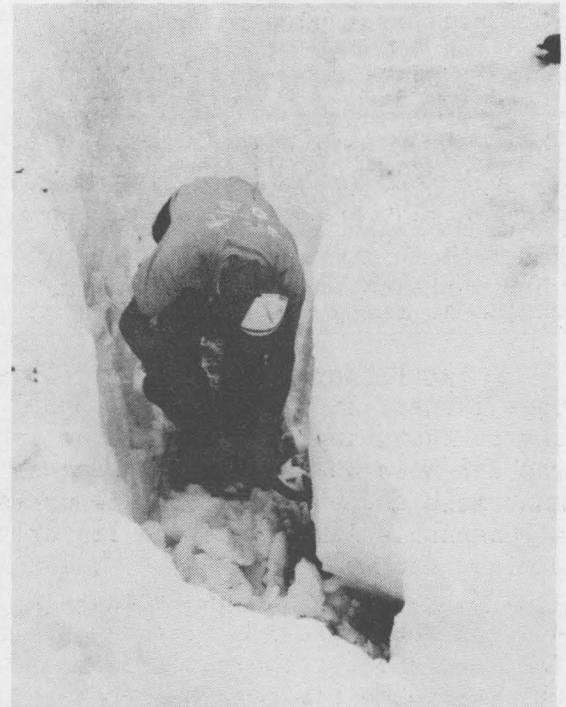
RECORD RECORDING — A surveyor digs out a "snow pillow" at the snow lab in June 1995. The 80-square-foot pressure detector bore 33 tons of snow in a late-melting accumulation that measured more than twice the normal amount.
